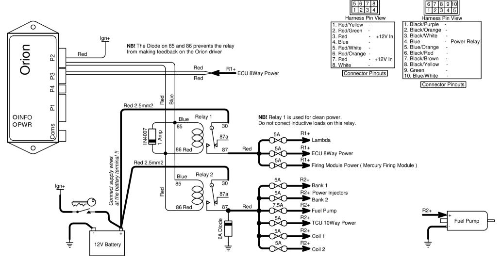
**NB!** Relay 2 is used for inductive loads. If you have more than 3 Coils use a third Relay to share the load. Try and keep Coils on their own relay. Add the 6 Amp Diode on to pin 87. It will prevent inductive spikes from the coils to damage lower voltage drivers of the injectors.
